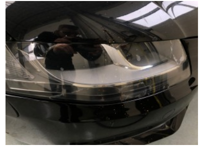
Right headlight - Weatherworn
